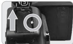
To unload the battery, tap the white knob and the battery pack will pop out.
