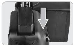
To load the battery, open the battery compartment cover. Push the Li-ion battery pack into the compartment according to the arrow indication. A white knob will lock the battery with a lock sound.
